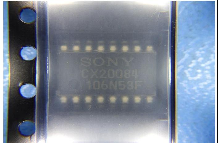
The carrier method used was 1 cut tape and reel containing a total of 17pcs. The manufacturing label displays related information about the components such as date code, lot code, country of origin, etc. P/N CX20084-T4 in this case was later found to be date code "0629", made in China, but the lot code was N/A.
